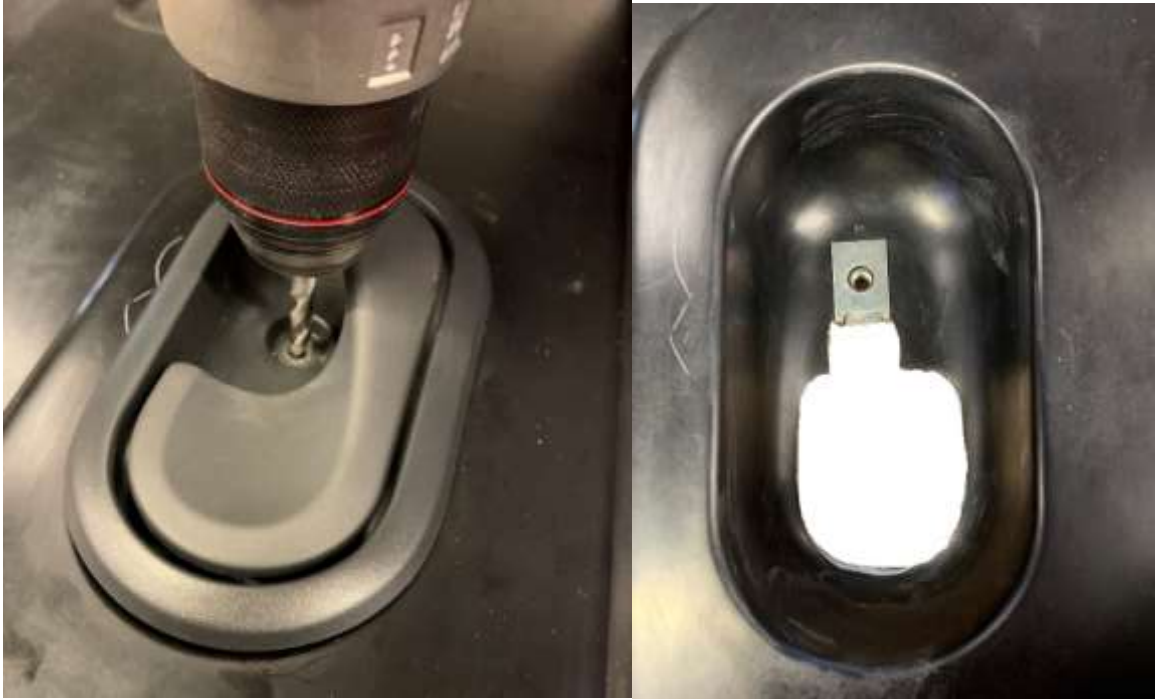
Figure 20: Drilling and door handle positioning
