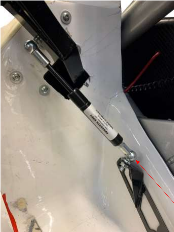
Figure 16: Damper assembly on door damper support bracket
